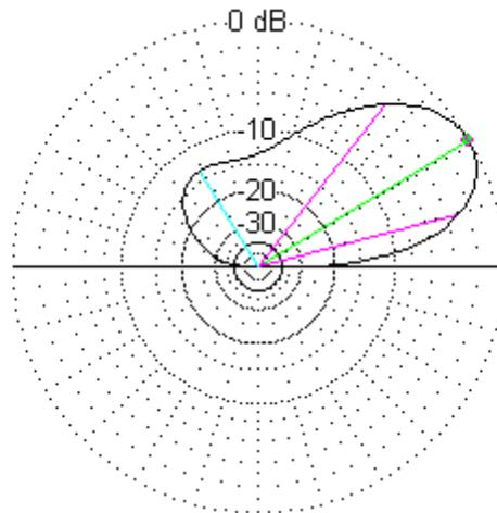
This plot shows EZNEC's guess of Tom's antenna pattern. His antenna was installed 60 feet above the ground. The front-to-back ratio I noticed on the air was better than what the graph above shows but variations in soil conditions, coax velocity factor, and other practical considerations could explain that difference. Tom had also said his the SWR was 1.7 to 1 or lower across the band.
