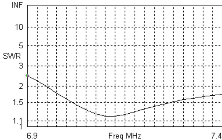
With a 25-Ohm matching section electrical length of 0.31 wavelength, the above SWR curve was achieved. This length provides a SWR under 1.6:1 across the entire 7.0 to 7.3 MHz band. That is clearly acceptable for amateur use. There is a caveat to this however. I expect that the matching section length need for individual installations will vary widely. This is the adjustment that will provide most of the compensation for variations in actual installations.
