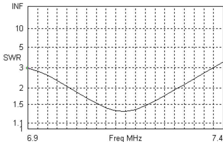
EZNEC's guess at the antenna's SWR curve was a little higher than Tom's measured values but this is often the case. Environmental factors often have large impacts on antenna feed impedances. Also, EZNEC does not include transmission line losses in its calculations. These losses tend to moderate SWR readings toward 1 to 1.
