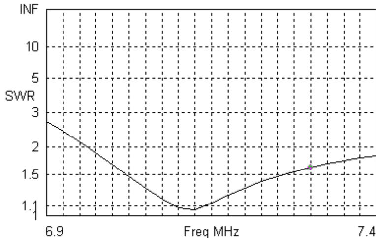
The plot above shows the SWR curve obtained by connecting an open stub of 50 Ohm coax at the transmitter end of the original quarter wavelength 25-Ohm matching section. In this case the stub needed turned out to be only about 8 feet long. The curve is not quite as good as what is available using Tom's method of adjusting the matching section length but it does point out that simple stub matching can be made to work.
