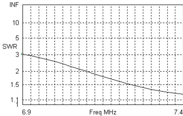
The SWR plot now looks like the plot above. It is better but still not nearly as good as Tom's antenna. I noticed that Tom specified a matching line section length that is not exactly  $\frac{1}{4}$  electrical wavelength long. Taking that as a hint, I tried adjusting the matching section length to see how it affected the SWR curve.
