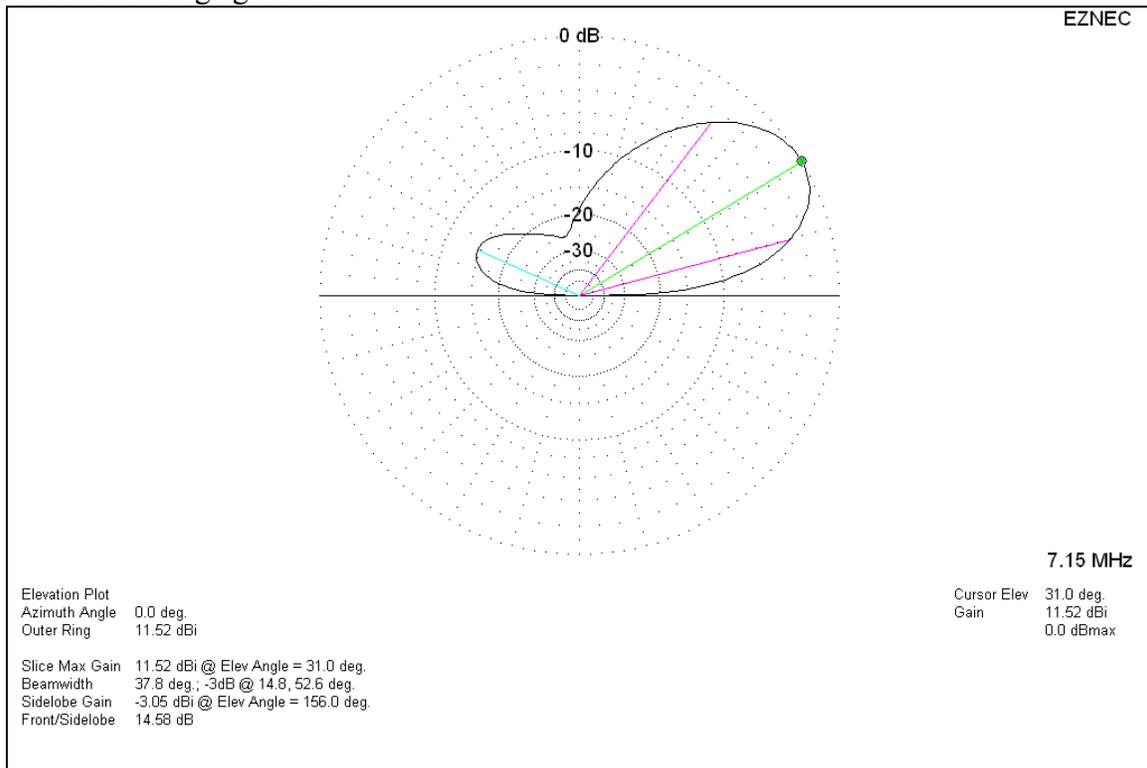
Keep in mind that the pattern above is for the original wire lengths and spacing. The optimum spacing for front-to-back ratio is actually a little less than a quarter wave, about 27 feet spacing for 40 meters.
