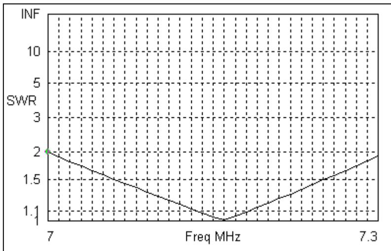
Reflector and director spacing was set to 27 feet from the driven element. Director length was 62 feet. Driven element length was 66.4 feet. Reflector length was 69 feet. Antenna height was set to 50 feet above EZNEC's average Real/High Accuracy ground
