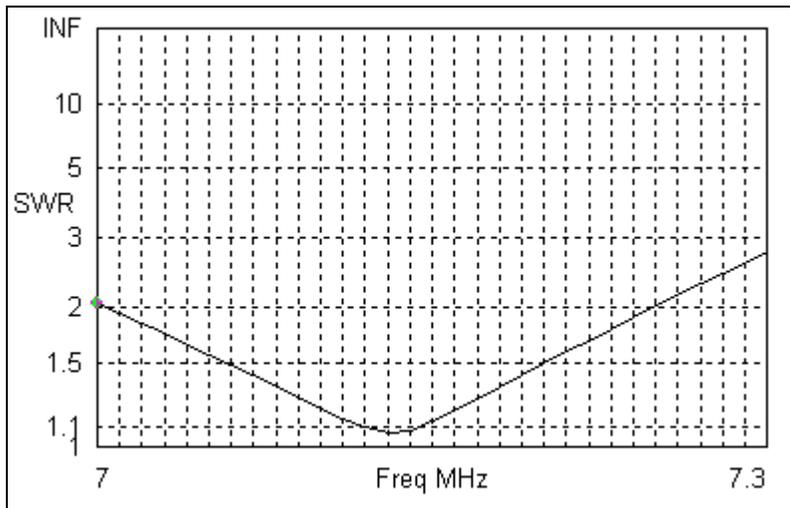
While examining variations on this antenna with EZNEC, I discovered that it is possible to find a combination of element lengths that will provide broadband 50 Ohm feed operation at essentially any equal element spacing value. Most interesting was that it was possible to achieve even better SWR bandwidth with closer spacing. With careful adjustment of director and driven element lengths, spacing down to and below 1/10 wavelength can provide good SWR bandwidth.
